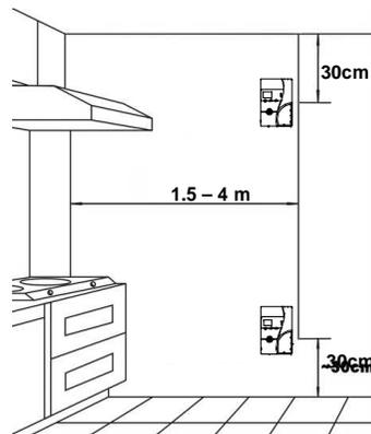
\*Ventilation hole showed as sketch , should be installed down.
